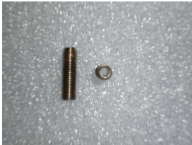
Figure 35. New fuel injectors developed for the use of gaseous fuels in AFIT's UCC sections.
