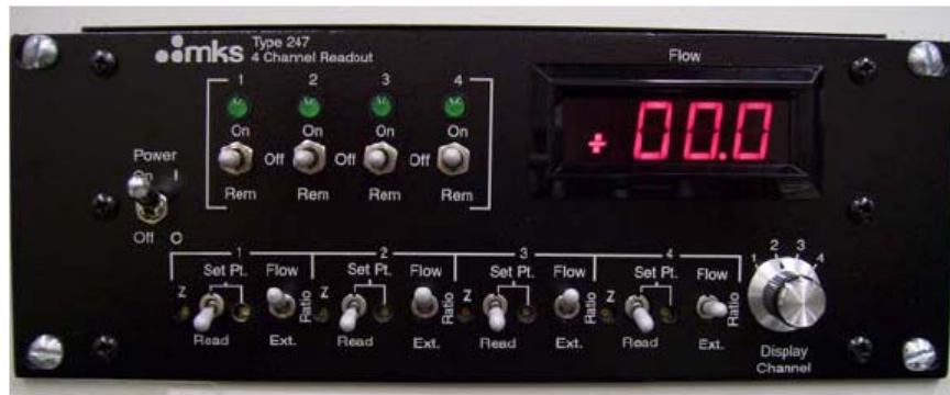
Figure 29. MKS Type 247 4-Channel Readout used to operate the MKS ALTA digital mass flow controllers (Hankins, 2008:49).
