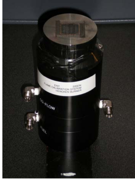
Figure 32. The Hencken burner used for calibration of AFIT's COAL lab laser systems.
