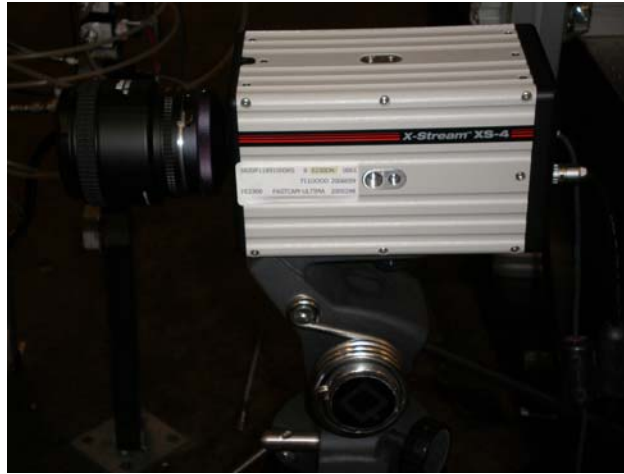
Figure 48. Integrated Design Tools, Inc. X-Stream XS-4 high-speed camera used for image collection in AFIT's COAL lab.
