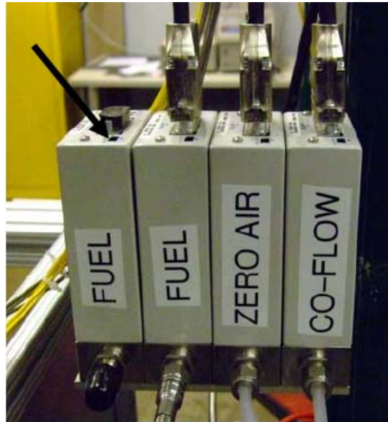
Figure 28. Several of the MKS ALTA digital mass flow controllers used in the COAL lab. The black arrow points to the zero reset button (Hankins, 2008:48).
