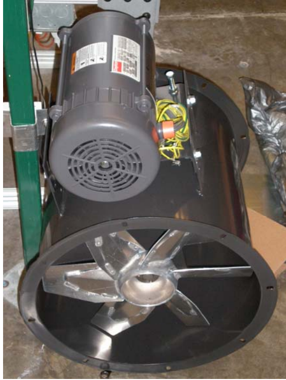
Figure 20. One of the 16” Dayton exhaust fans.
