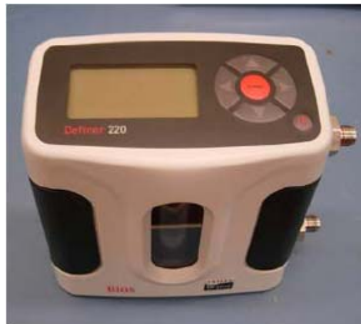
Figure 30. BIOS International Corporation Definer 220-H flow meter used for calibration of the MKS ALTA digital mass flow controllers (Hankins, 2008:50).
